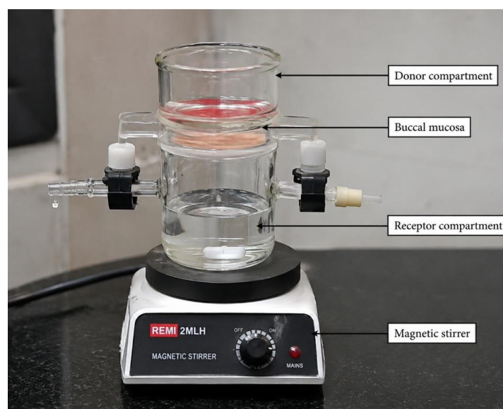
Figure 4: Franz Diffusion Cell Setup for Ex-vivo Buccal Permeation Study.
